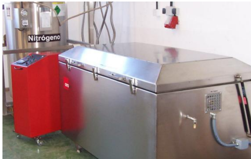
Figure-[1.3] Multistage cryogenic processor[20]
